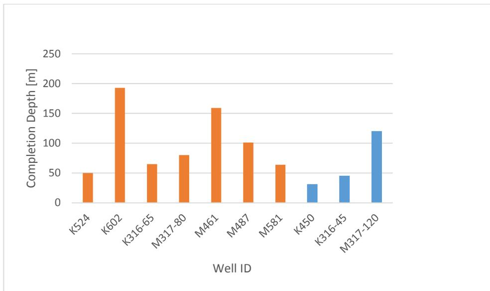
**Figure 12** Completion depths for 10 boreholes in Kilimanjaro and Manyara. Alluvial aquifers are shown in blue, and fractured bedrock aquifers are shown in orange.
